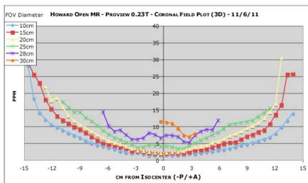
The plot immediately below shows the spherical homogeneity prior to the reshim and at two subsequent visits.
