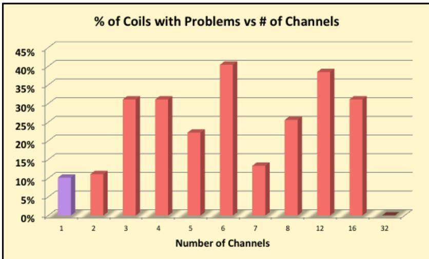
From the summary table above, we see that there is little difference in one and two channel coils, roughly 10% have some sort of problem. 25% of all multi-channel phased array coils have a problem. If you ignore the two channel coils then the % of coils with a problem goes up to 28%. Unless the physicist looks at each channel, many of these problems will be missed.
